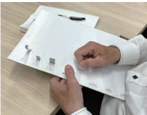
The team tested perforated tear-off strips over and over again to find the optimum thickness, angles, and toughness.
