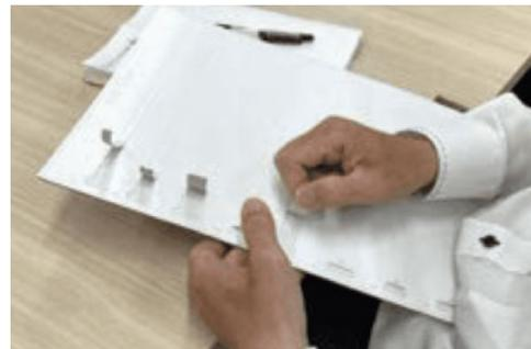
**The team tested perforated tear-off strips over and over again to find the optimum thickness, angles, and toughness.**
