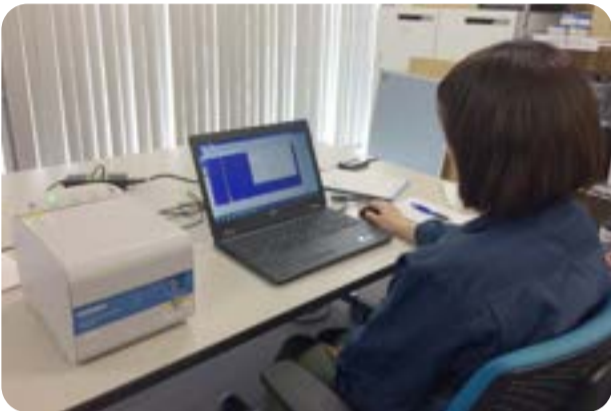
Scanning for heavy metals using X-ray fluorescence
