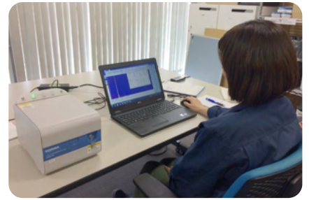
Scanning for heavy metals using X-ray fluorescence (KOKUYO Head Office)
