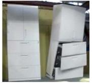
Equivalent to the intensity 6 upper level Left: With wall fixtures Right: Without wall fixtures
