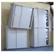
Equivalent to the intensity 5 lower level Left: Without connectors Right: With connectors
