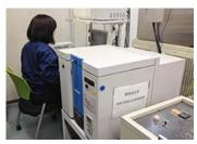
Checking for the presence of heavy metals using an X-ray fluorescence spectrometer
