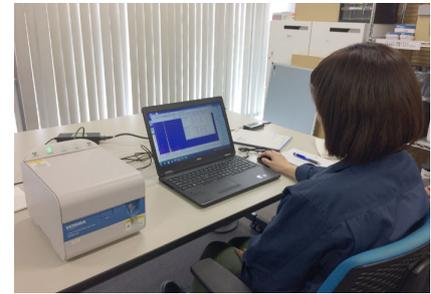
Scanning for heavy metals using X-ray fluorescence
