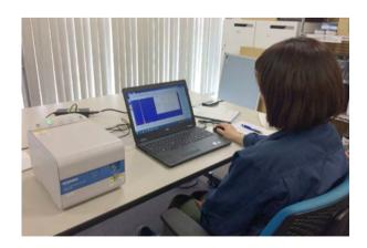
Scanning for heavy metals using X-ray fluorescence
