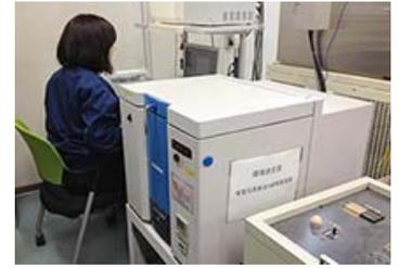
Checking for the presence of heavy metals using an X-ray fluorescence spectrometer.
