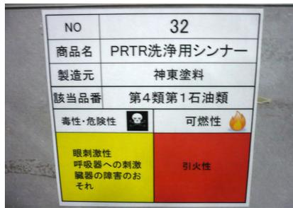
Color coded sections on label communicate hazards (Shibayama Plant)
